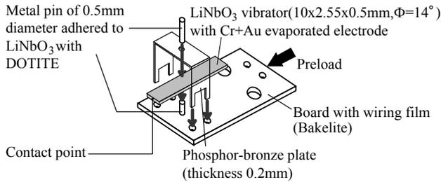
Fig. 12. Support configuration of stator vibrator.
