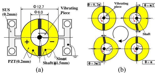
Fig. 1. (a)Construction of a stator vibrator and (b) vibration mode and operating principle.
