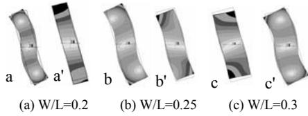
Fig. 11. Resonant vibration mode displacement at  $\Phi=15^\circ$ .
