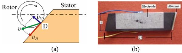
Fig. 5. (a)Operating principle of the trial motor and (b)photo. of its stator vibrator.
