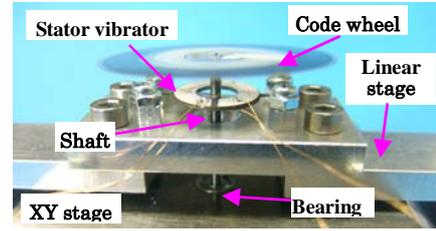
Fig. 2. Measurement apparatus of the ultrasonic spindle motor using an annular plate-type vibrator.
