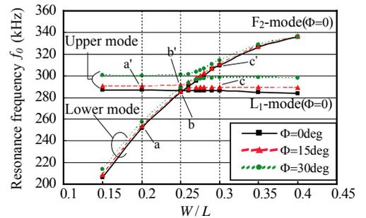
Fig. 10. Analysis result of the resonance frequency correlate with the width-to-length ratio  $W/L$ .
