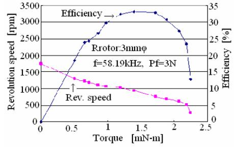
Fig. 8. Load characteristics. (Lower-mode, Rotor diameter: 3.0mm).
