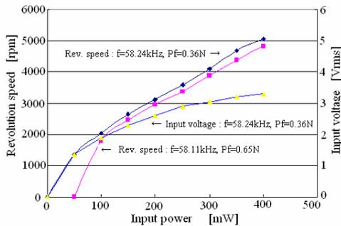
Fig. 7. Characteristics of the motor. (Lower-mode, Rotor diameter: 1.5mm)
