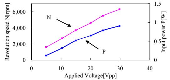
Fig. 3. Measured results of revolution speed and input power to applied voltage.
