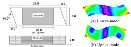
Fig. 4. Diagonally symmetrical multilayer ceramic vibrator and its vibration modes by FEM.
