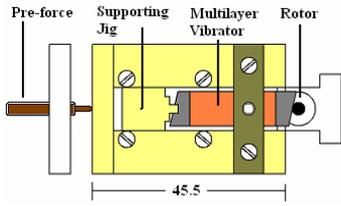
Fig. 6. Trial motor construction.
