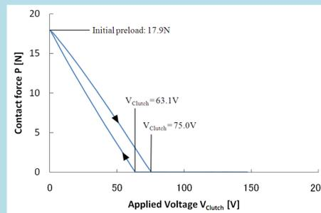
**V<sub>clutch</sub> = 75.0V:** The head of the USM was separated from the load cell.
