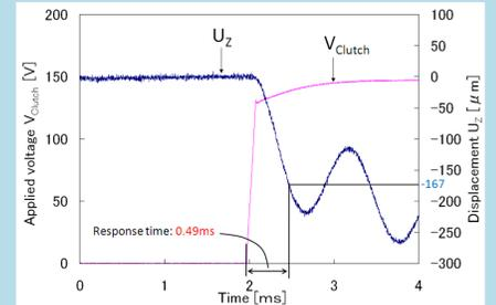
Fig. Measured response time of displacement at the point O immediately after input pulse.
