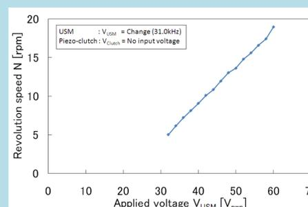
Fig. Revolution speed vs. input voltage to MPAs of USM.
