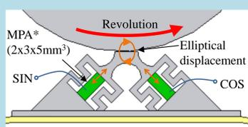
Fig. Operating principle of the USM.
