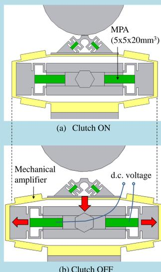
Fig. Operating principle of Piezo-clutch.
