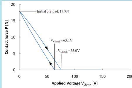
$V_{clutch} = 75.0V$ : The head of the USM was separated from the load cell.
