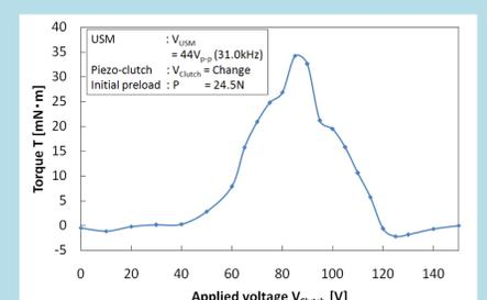
Fig. Torque vs voltage applied to MPAs of piezo-clutch.
