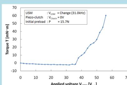
Fig. Torque vs voltage applied to MPAs of USM.
