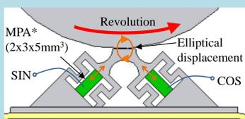
Fig. Operating principle of USM.
